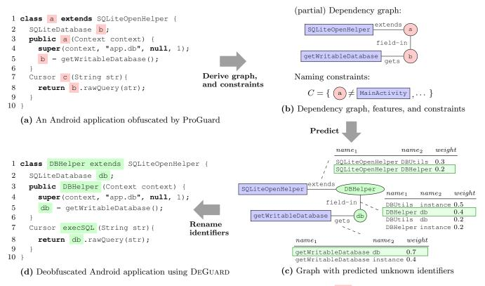
Figure 1: Statistical deobfuscation of Android applications using DEGUARD. The red color indicates the elements whose names are to be renamed (in the input), the green color are the same elements with the new names (in the output), and the purple color denotes the elements whose names are known and remain the same.
